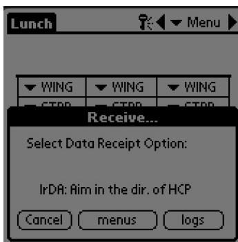
Figure 2: To download a cabinet's configuration, hold the Palm parallel to the floor and a foot away from the cabinet's lens in the top right corner. Tap the RX Mnems button. To download a log of daily activity, tap the Rx logs button. A dialog box will display after the transfer is complete. Button names on later software versions may vary from what's shown above.
