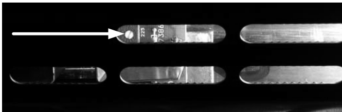
Figure 2: The potentiometer, indicated by the arrow, is adjusted using a narrow-blade screwdriver.
