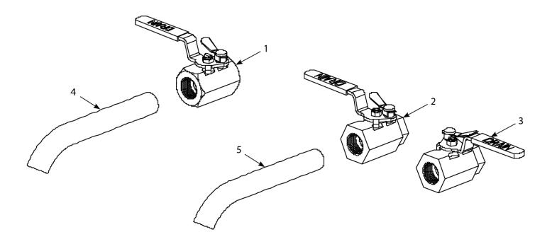
Drain System Components - Drain Valves and Associated Parts (Units without Built-In
