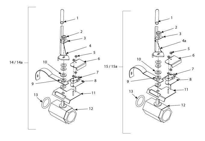
Drain System Components - Drain Valve Assembly and Assoc.Parts (Units
