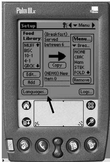
Figure 1: Arrow points to the Language button, where the temperature display and the language displayed can be altered.
