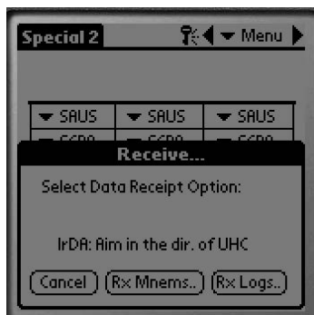
Figure 2: To download a log of daily activity, tap the Rx logs button. A dialog box will display after the transfer is complete. Button names on later software versions may vary from what's shown above.
