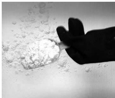
Use a measuring cup or scoop to evenly distribute filter powder over the filter sheet.
