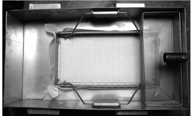
Properly assembled filter pans, ready for use.
