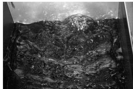
Bubbling oil indicates that air is flowing through the return lines and all oil/shortening has been evacuated from the lines.
