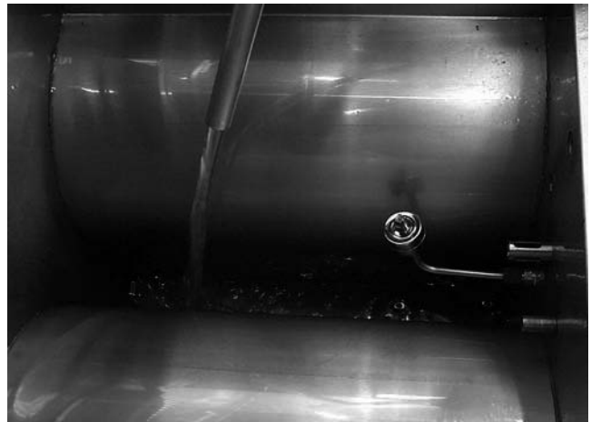
Use the nozzle to rinse sediment and debris from the frypot during the filtering process ("U" units only).
