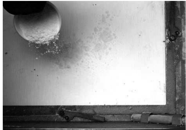
Evenly distribute 8 ounces of filter powder over the filter paper surface.
