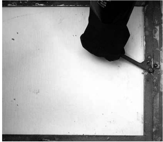
Secure the hold-down ring latches to lock filter paper in place.
