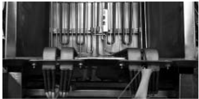
Thread probe wire through hole in tilt plate assembly, then remove probe and components from element.
