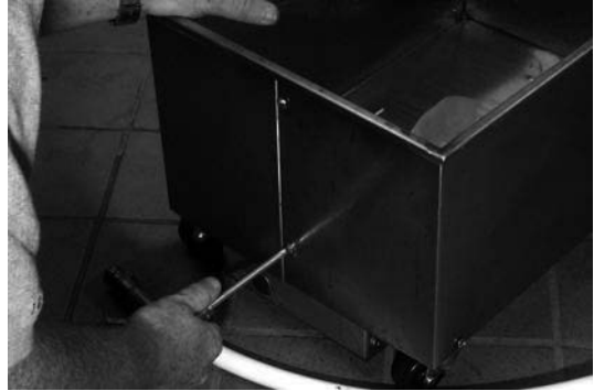
Remove screws securing outer panels.
