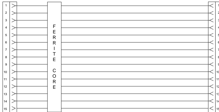
8121353 CONTROLLER CABLE 15-Pin Male Connectors on 5-Foot Shielded Cable (Ferrite Core at Controller End)
