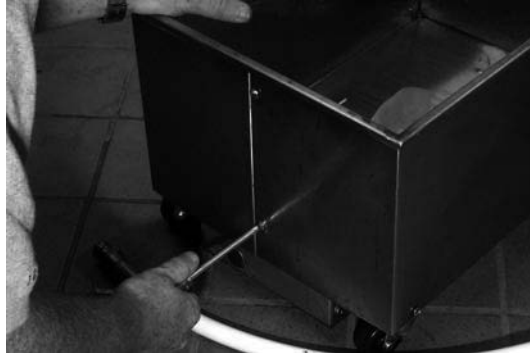
Remove screws securing outer panels.
