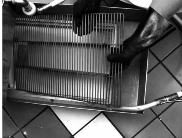
Removing paper support screen from pan.
