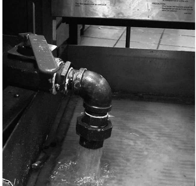
Frypot draining into filter pan. Ensure oil is at operating temperature before opening drain valve.
