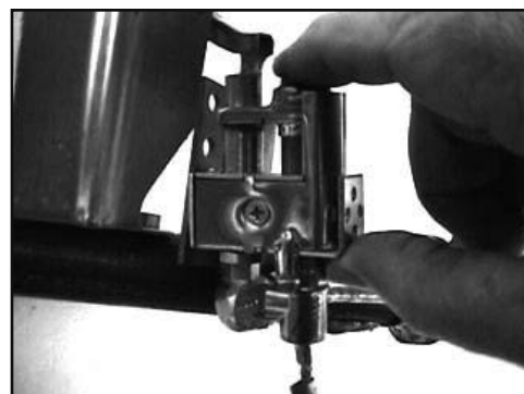
Bend the clip to release the thermopile.
