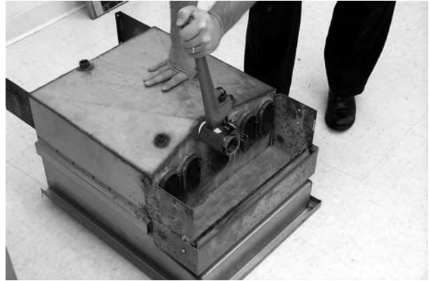
Removing drain valve from frypot.
