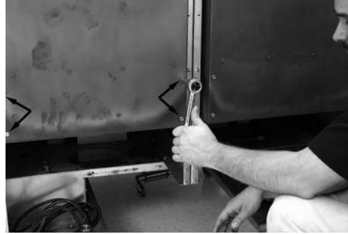
Removing bolts (arrows) securing flue to frypot.
