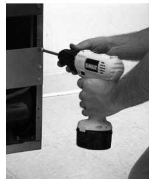
Removing gas manifold shield.
