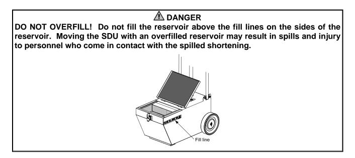
4. Carefully withdraw the unit far enough to allow the cover to be closed. Latch the cover in the closed postion. Using the handle, carefully tip the unit back slightly for ease of handling and roll the unit to the disposal site.
