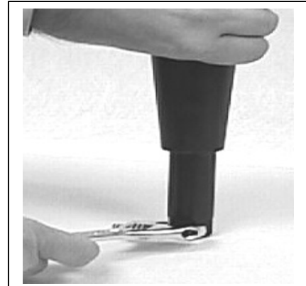
ADJUST LEG HEIGHT WITH AN ADJUSTABLE WRENCH
