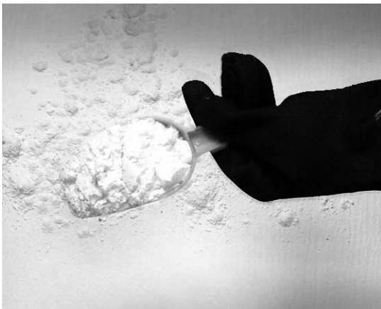
Applying filter powder to filter paper.
