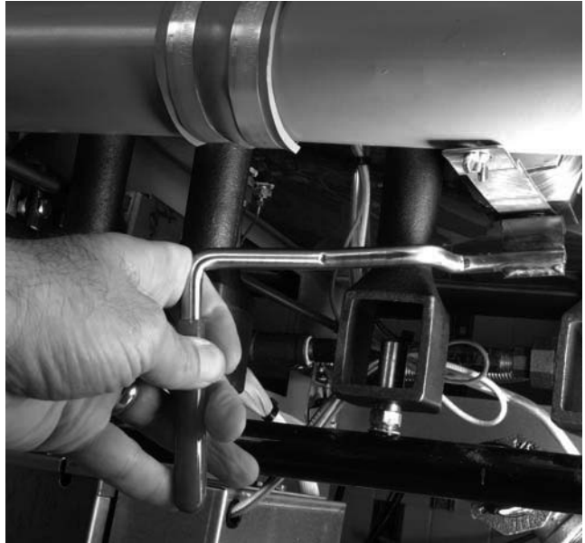
Move the red drain valve handle into the open position.
