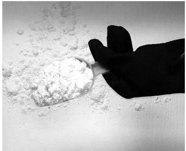
Applying filter powder to filter paper.
