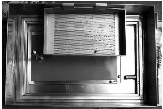
Crumb screen properly placed in filter pan.
