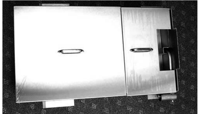
Pan covers properly placed on filter pan.
