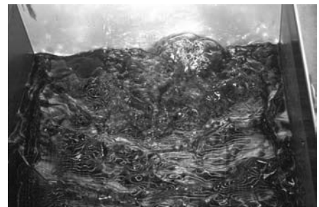
Air bubbles from the Oil Return Line
