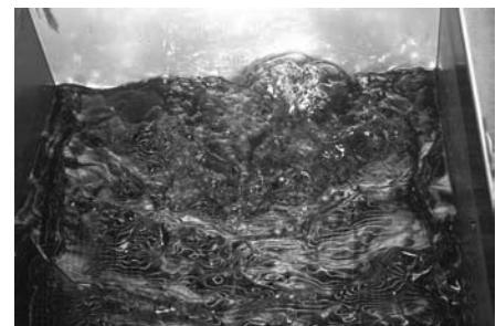
Air bubbles from the Oil Return Line
