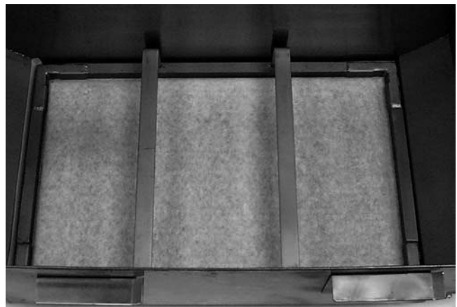
Hold-down ring positioned correctly over filter paper in filter pan.
