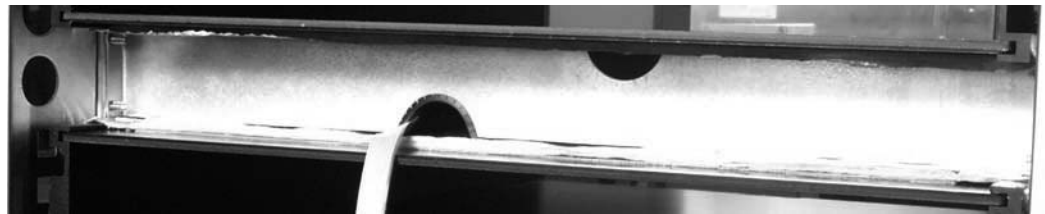
Figure 10: A baffle is secured behind the bezel.
