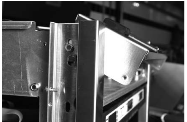
Figure 3: Remove the screws which secure the component shelf, allowing the shelf to be pulled forward.
