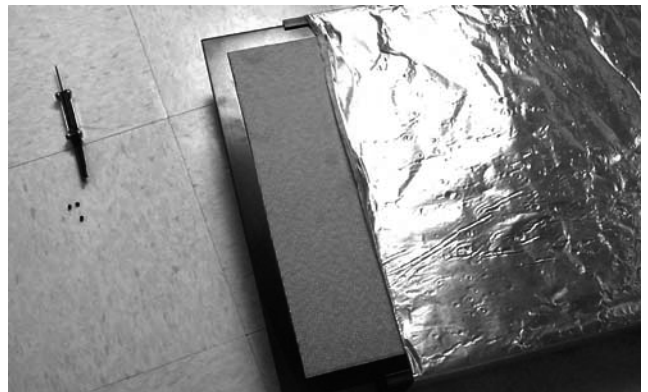
Fig. 13: The heater plate slides from the insulation.
