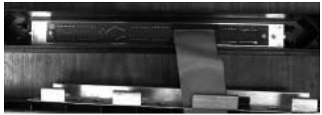
Fig. 8. Note ribbon cable is at top of bezel opening.
