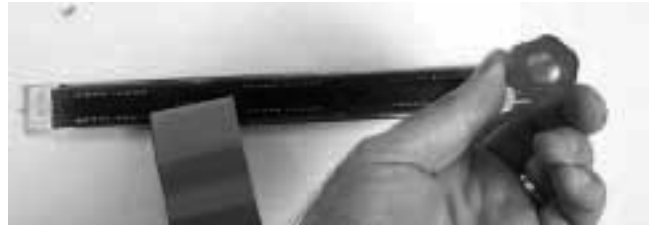
Fig. 9. Remove two screws securing the display board to the membrane switch.
