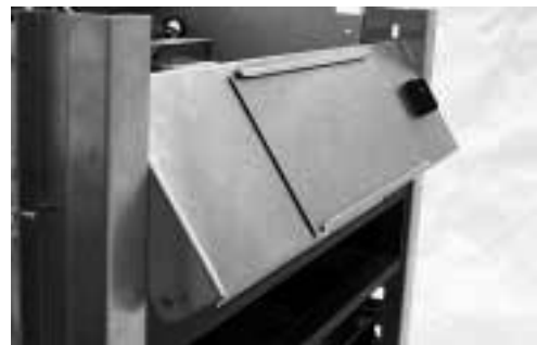
Fig. 3. Removing front fascia.
