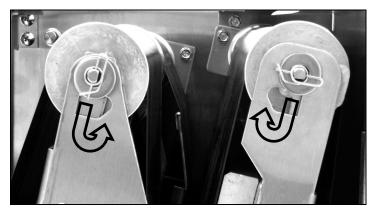
5. Rotate the tray stabilizer latch upward to unlatch it.
