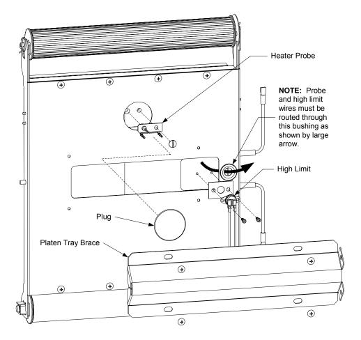
4. Replace the failed component, being sure to route the component wires through the bushing as shown in the illustration above. Reassemble by reversing the steps performed and reconnect the wiring in accordance with the wiring diagram on the inside of the component housing cover.
