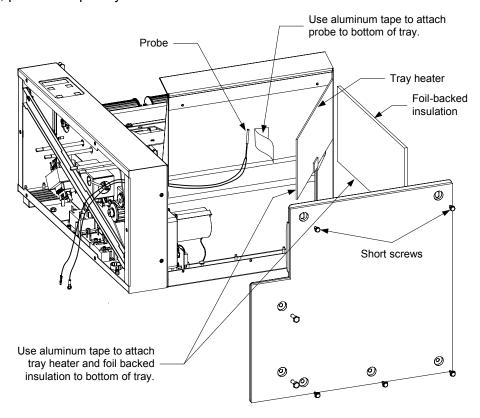
9. Reverse the steps performed to reassemble unit.
