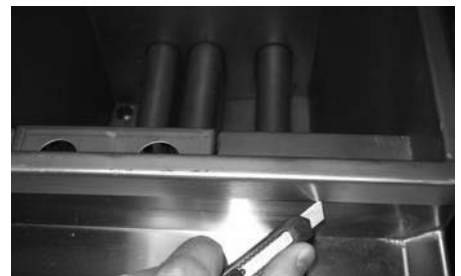
Cut cookpot seal prior to cookpot removal.
