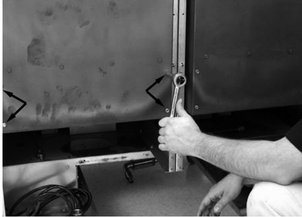
Removing bolts (arrows) securing flue to cookpot.
