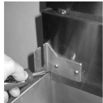
Removing flue cap.
