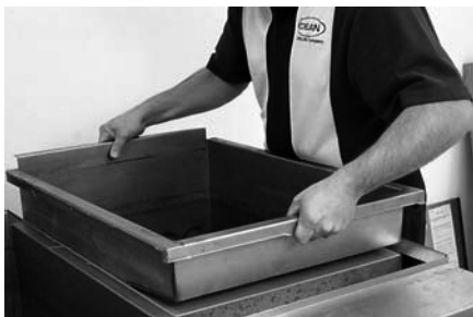
Lift cookpot from rethermalizer.
