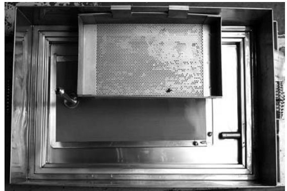
Placing the crumb screen.
