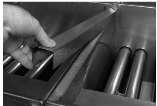
Removing the joiner strip.
