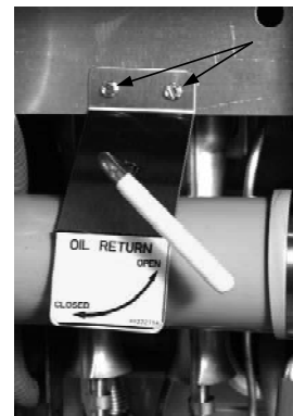
Oil-return handle bracket and screws.
