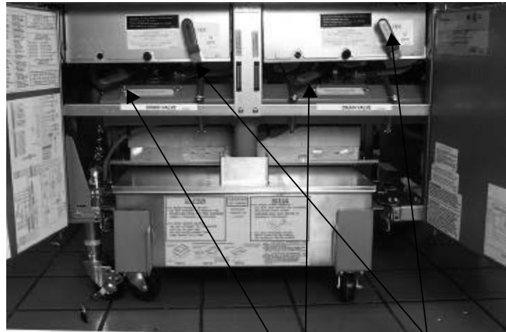
Fig 12-14 Handles used during filtering: Drain valves
