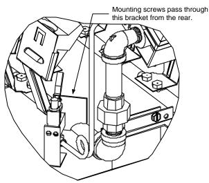
On GF40 units, the pilot and thermopile assembly is attached to its mounting bracket by two screws that pass through the bracket from the rear. The burner assembly should be removed to access these screws.
