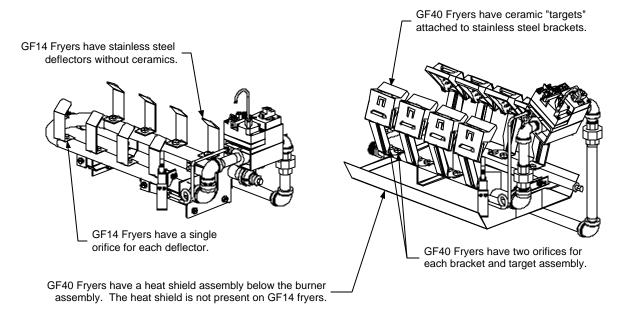
The flames originate from orifices in a U-shaped burner manifold positioned beneath the frypot. The orifice diameters differ for natural and Propane (LP) gas and for fryers as indicated in the accompanying table (NOTE: This table shows only the orifices used in elevations up to 1999 feet/609 meters. See Chapter 2 (GF14) or Chapter 3 (GF40) for orifices required at other elevations). GF14 fryers have one orifice per deflector; GF40 fryers have two orifices per deflector assembly.
