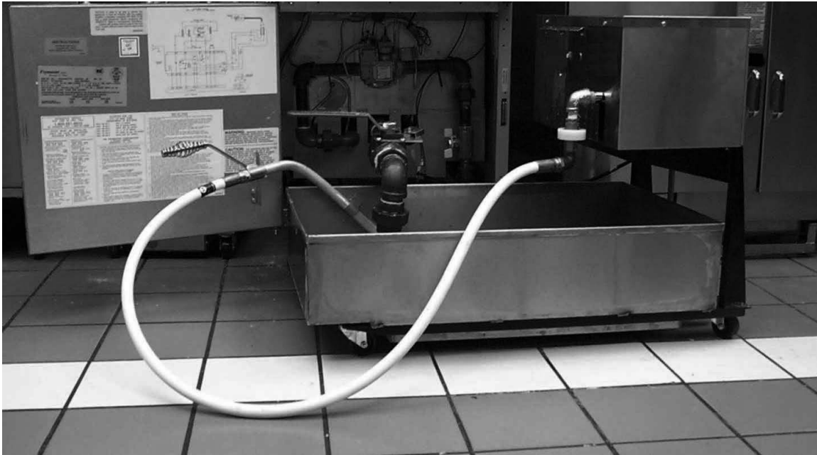
MF-90 portable filter (Low Profile shown) positioned correctly next to fryer drain valve, with rear casters locked in place.
