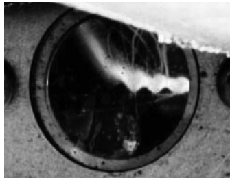
Lifting flame with too much air
