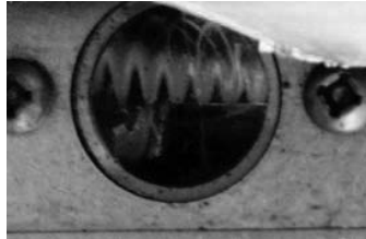
Lifting flame with lack of air
