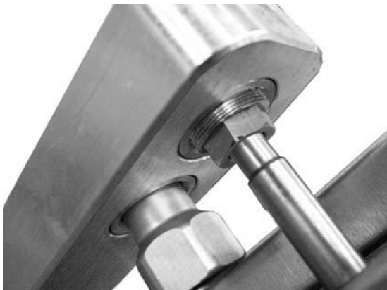
Figure # 7 - No more than two (2) threads male, as per diagram showing above
