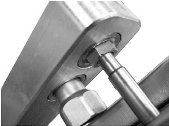
Figure # 6 - Desired position, both threads flush, as per diagram showing above
