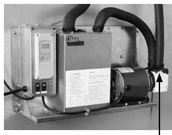
Connect glycol recirculating line from pump outlet 3/8" barb fitting to the beer line set.
