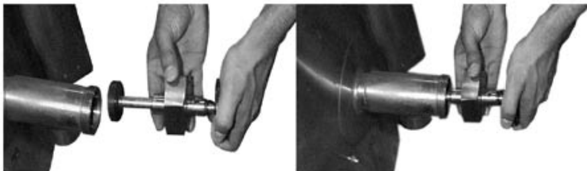
Assemble and attach the tangent draw-off valve after the kettle is unpacked.
