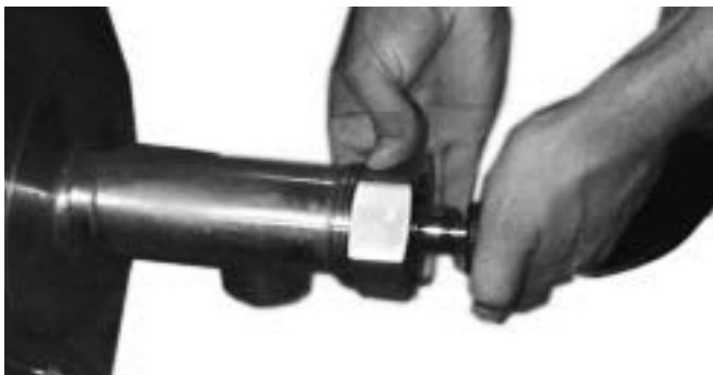
When attaching the draw-off valve hand-tighten the nut.
