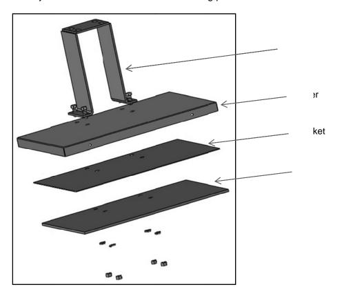
1.4 Align the holes in the riser bracket to the cover as shown and install the mounting bolts, lock washers and nuts to secure the bracket to the cover, gasket and backing plate. Tighten the nuts to a 20 ft/lb torque with a 3/8" open end or socket wrench.
