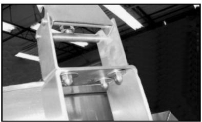
2.2 Assemble the actuator to the three studs on the domed cover and secure using thread locking compound and the dome nuts supplied in the cover kit. Tighten the dome nuts to 20 in/lb torque with a 1/4" open end or socket wrench.
