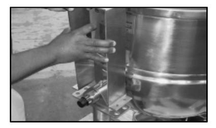
1.4 Align the holes in the riser bracket to the cover as shown and install the mounting bolts, lock washers and nuts to secure the bracket to the cover, gasket and backing plate. Tighten the nuts to a 20 ft/lb torque with a 3/8" open end or socket wrench.
