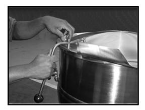
2.6 Adjust the tension in the actuator assembly by turning the adjusting nuts as shown. Use two 3/4" open end wrenches.
