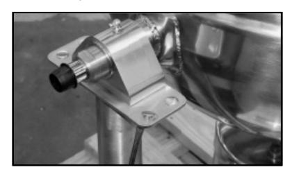
1.3 Align the riser to the holes in the trunnion plate as shown.
