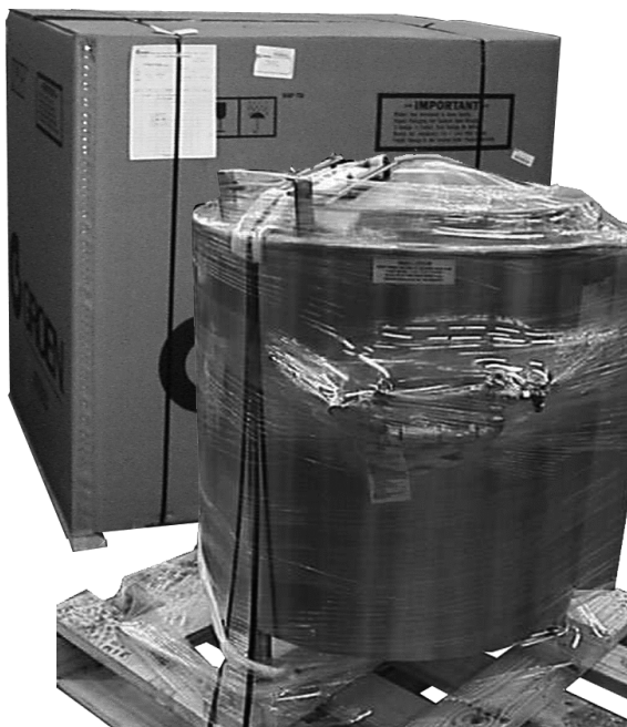
The kettle will be banded to a skid, inside a heavy carton.
