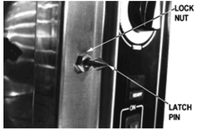
Adjust the door latch pin to allow for changes that might occur as the gasket ages
