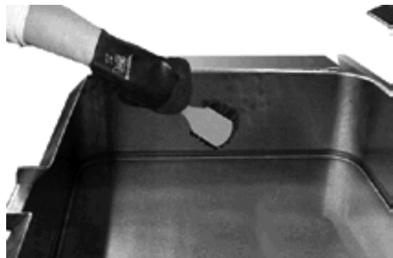
Use a brush, sponge, cloth, plastic or rubber scraper, or plastic wool to clean.
