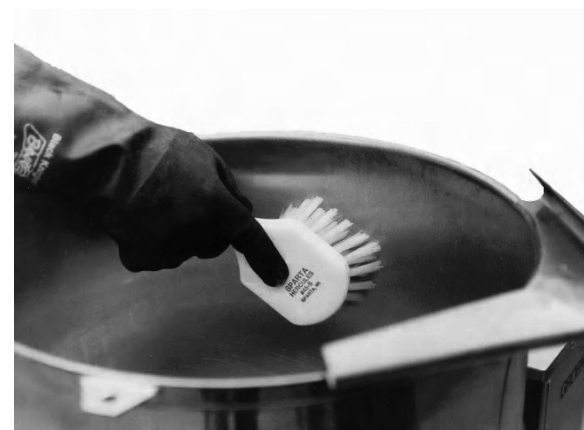
Use only a sponge, cloth or plastic brush to clean the kettle.
