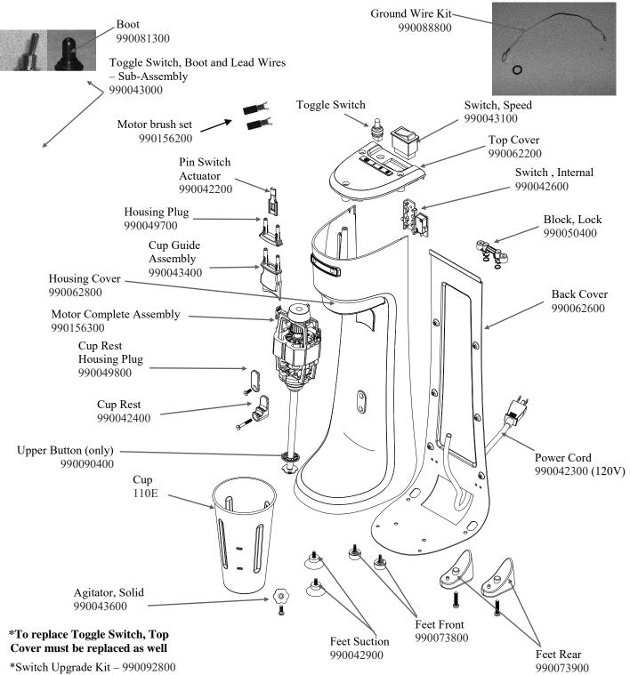
Includes: Upper Lid, Toggle Switch, Boot, Grounding Wire, and Switch Adaptor
