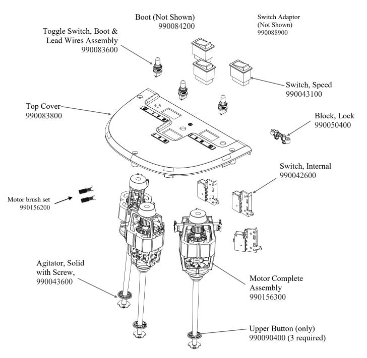
\*Switch Upgrade Kit for series A-D – 990092900 Includes: (1) Top Cover, (3) Toggle Switch, (3) Boot, (3) Grounding Wire, and (3) Switch Adaptor
