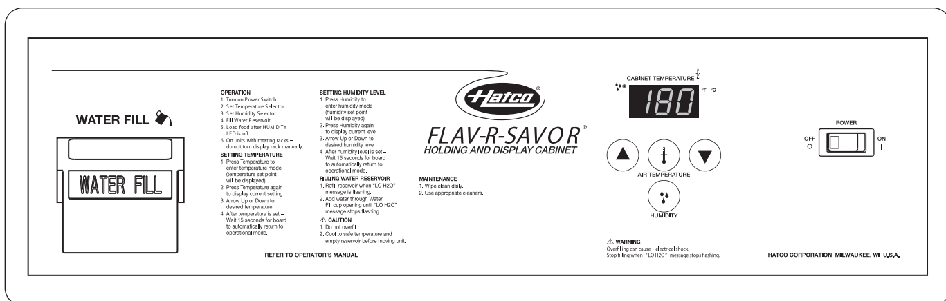
Figure 9. FSD/FSDT Control Panel
