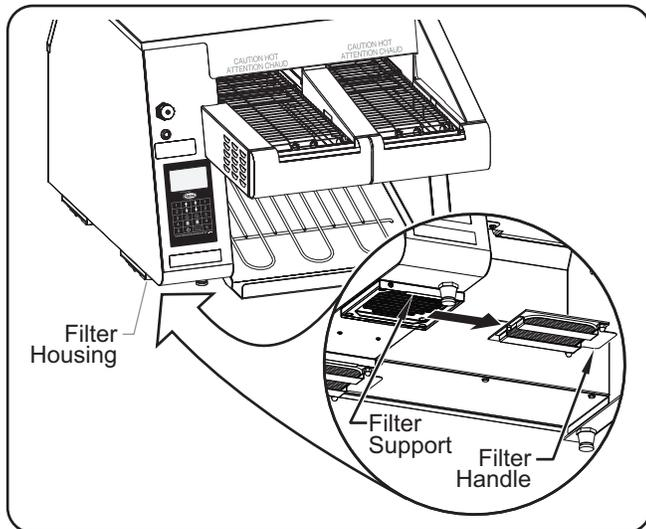
Removing/Installing the Filters
