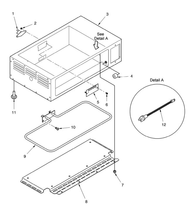
Figure 2-2. Heater and High Limit
