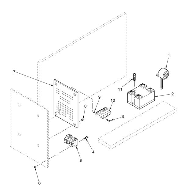
Figure 2-4. Electrical Parts
