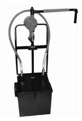
8. Swivel pump assembly over disposal container and tighten thumb screw on bracket.
