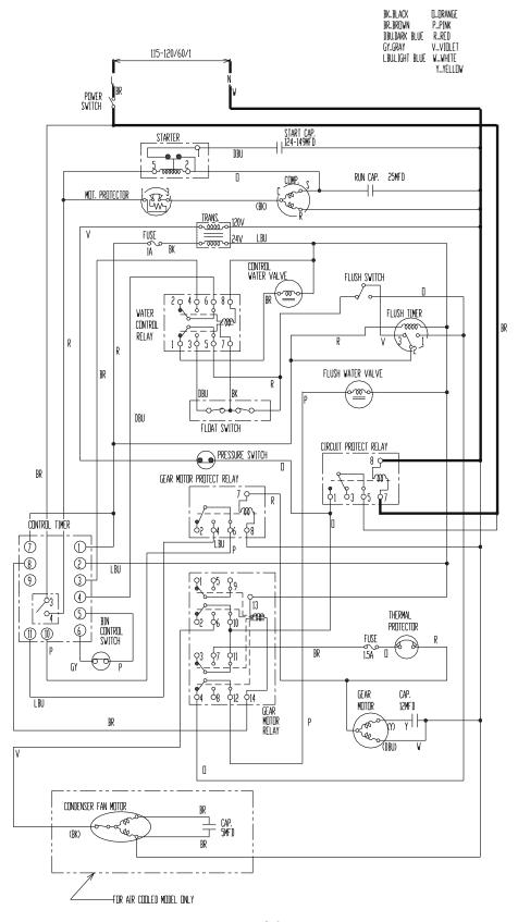
[j] When input voltage is too low, (Less than 70%), Gear Motor Fuse (1.5A) is blown causing the Compressor and Gear Motor to turn off immediately.
