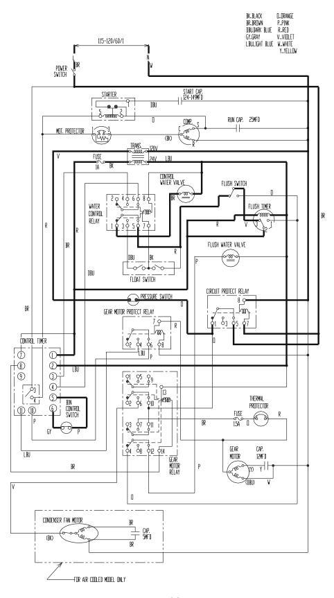
[f] Low Water (Water-cooled Model), or Dirty Air Filter (Air-cooled Model), Pressure Switch to "OPEN", Compressor and Gear Motor operates intermittently.
