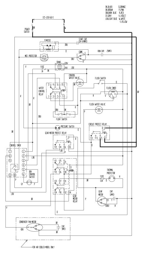
[g] When Flush Switch is moved to "FLUSH" position, Flush Water Valve opens and flushes Reservoir and Evaporator.
