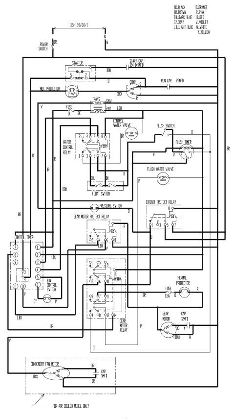
[d] Bin Control operates, and about 6 sec. later, Compressor and Gear Motor stop simultaneously.
