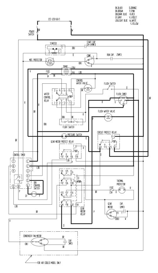
[i] When 208-230V are supplied to Circuit Protect Relay, it protects the circuit from miswiring. If the power supply is properly connected, the contact of Circuit Protect Relay does not move even when the coil is energized.
